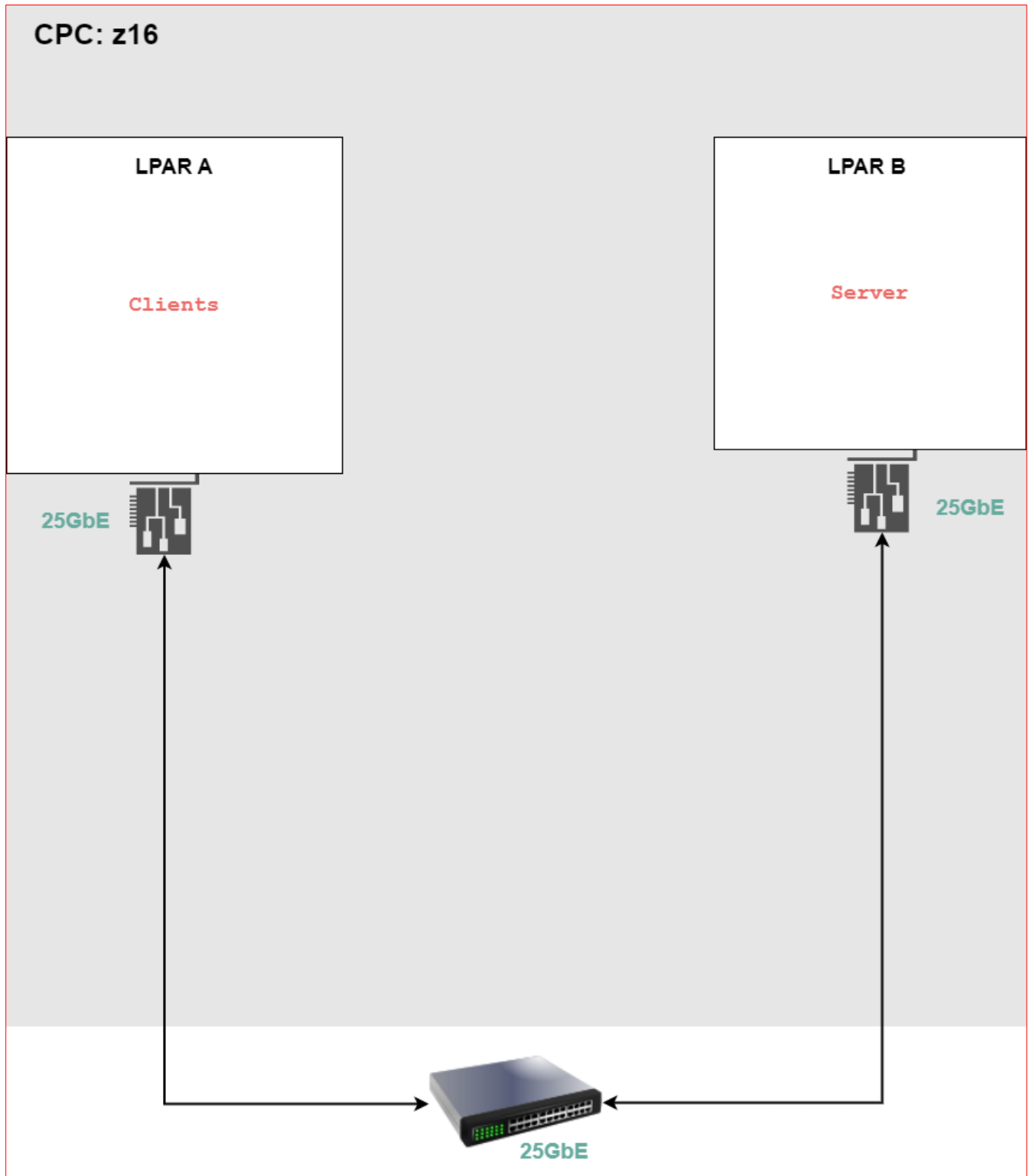
Figure 9: Test set-up where the clients and server run natively on z/OS UNIX
