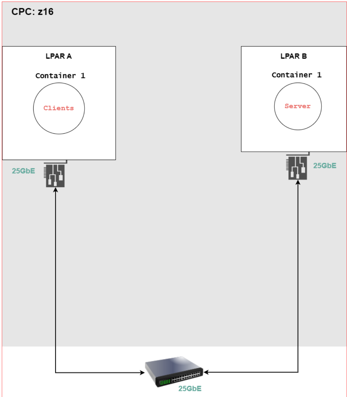
Figure 10: Test set-up where the client & server are containerized
